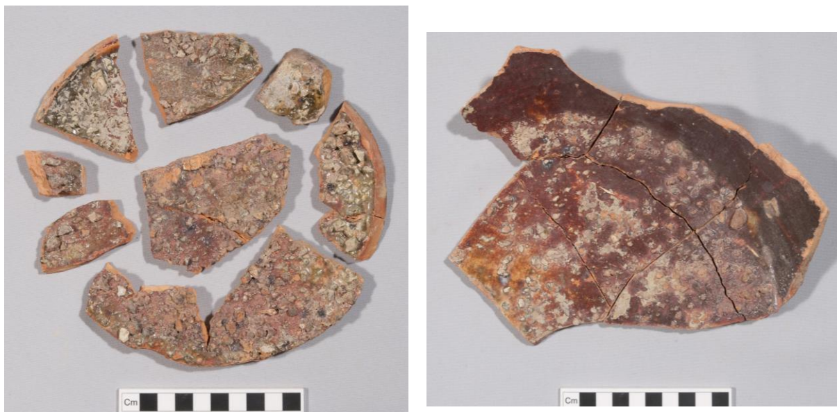
Figure 4.91: Evenly encrusted base setter fragments, left 7646/85026 and right 7646/85006. Russell Workman, 10cm scale.
