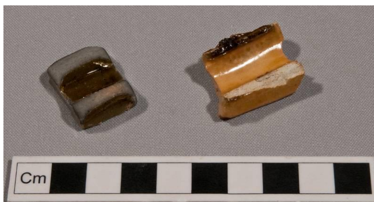
Figure 4.79: Spurs Type 12.3.1 with dripped/pooled glaze and ridges broken off from adhering vessels (left-right: 7645/88575, 88576). Russell Workman, 10cm scale.
