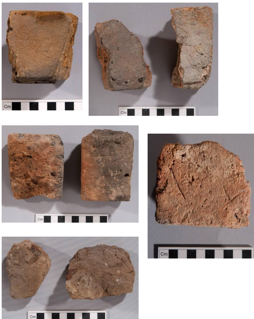
Figure 4.50: Shaped and marked bricks from the kiln structure found in context 7460. Top row left: corbel or keystone brick (95298). Top right and Middle row left: bricks with bevelled side edges and partly darkened dense clay fabric (95208). Middle row right: brick fragment with incised 'XX' tally mark (95195). Bottom: dense brown clay bricks fragments (95212). Russell Workman, 10cm scale.
